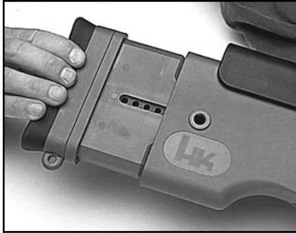
Figure 35 Remove buttplate with spacer
