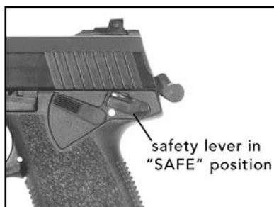
Figure 4 "Safe" Position (hammer cocked)
